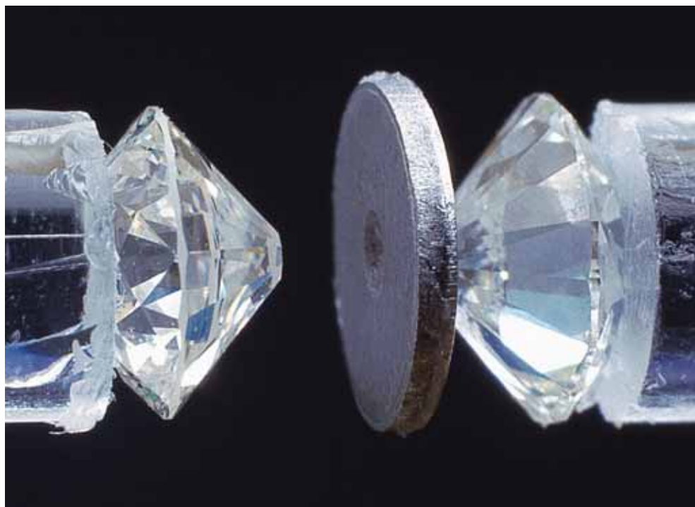
Two diamonds are used to press together samples of rock and iron at a pressure of 1 million atmospheres. A laser then heats the sample to 5000°C. Only the test samples heat up.
