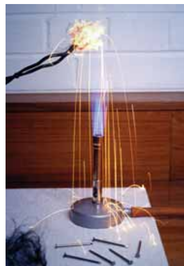
Figure 2.3 Oxygen is very reactive. Under the right conditions, it can cause steel wool to burn.
