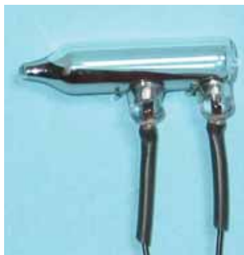
Figure 2.7 The switch turns on when the mercury flows over both wire leads, making an electrical connection. When the tube tilts, the connection is broken, and the switch turns off.
